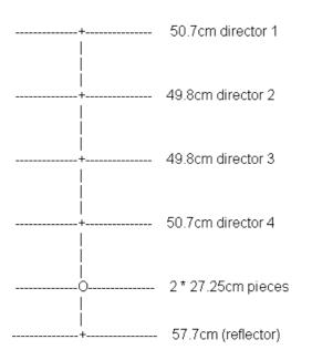
All element spacing are taken from the reflector to the element in question.
